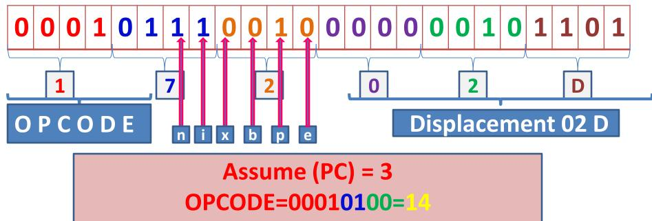
OPCODE=00010100=14 Format = 3 n i = 1 1 (DIRECT ADDRESS) P=1 EA= (PC)+ Displacement =003+02D=0030 http://cis.csuohio.edu/~jackie/cis335/sicxe\_address.txt
